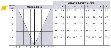
Note: If using No. 11 honeycomb baffle multiply footcandle values by .80
